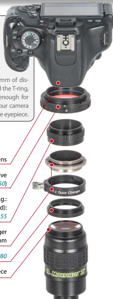
Cameras with a fixed lens and a filter thread can also be combined with the Morpheus® eyepieces. The lens should be close to the eyepiece, without touching it. Our DT-rings come with a 1 mm spacer ring, to enable you to fine tune your camera's position to be as close to the eyepiece as possible without contacting the eye lens. Use the camera zoom, until the black frame around the image disappears – a tele lens is better than a wideangle lens.
