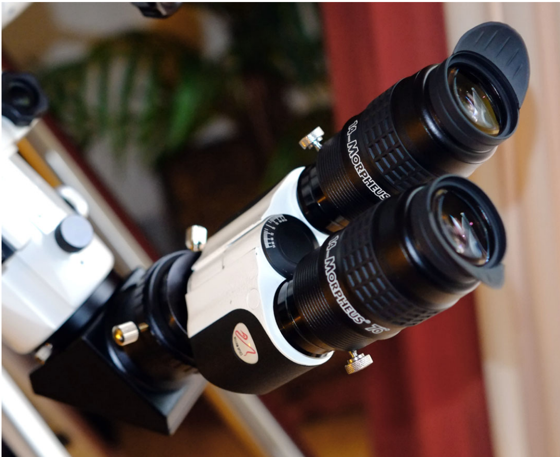
Fig 10: 14mm Morpheus eyepieces with included optional winged eyeguards in a William Optics binoviewer.
