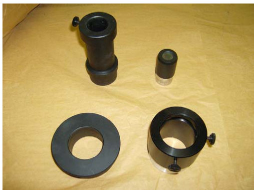
Figure 2: Here are the standard accessories used for collimation and setting the primary to secondary distance for the CDK12.5 and CDK20.
