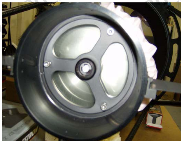
Figure 6: CDK20 secondary housing. There are three collimating screws and a central knob. The secondary is spring loaded pulling the secondary into the three collimating screws.
