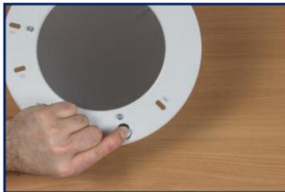
**3.3.6** Keep your fingertip on the head of the M4 Phillips screw to avoid it from rotating while fastening the bolt.
