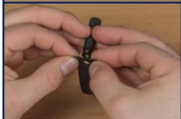
Make sure that the side of the strap which has the double-sticky tape on it faces the table while applying it to the bolt.
