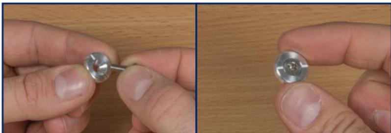
3.3.2 Place black sliding washers in parallel to the milled surfaces on the lower part of the sliding fastener
