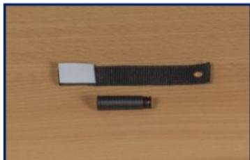
Prepare the supplied bolts on a table and attach the Safety Straps to the bolt by pressing the hole in the strap onto the upper side of the bolt until it rests in the depressed area in the bolt.
