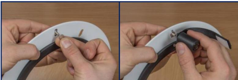
**For other bolts:** Fasten the supplied bolts with the safety straps already attached (see 3.2) at the M4 thread on the opposite side without additional washers in between.
